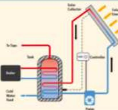
Solar panels made up of evacuated tubes or flat-plate collectors **heat up water stored in a tank**. The energy is used for hot-water supply and, occasionally, space heating.
