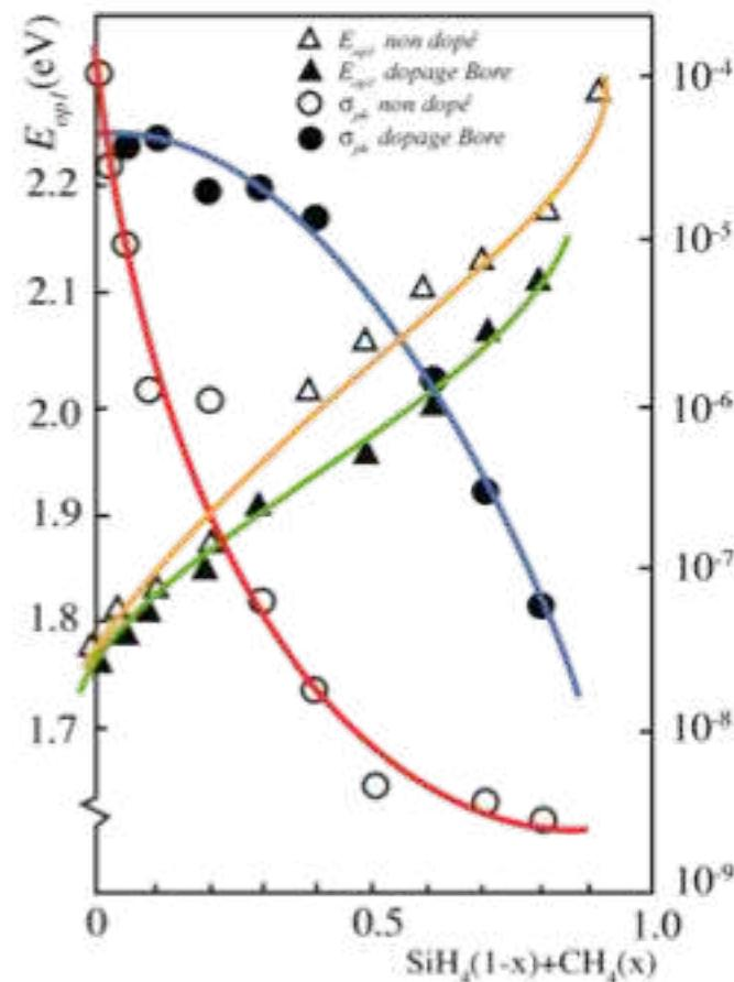
Ability to vary the gap between 1.0 and 2.2 eV, from a gaseous mixture (plasma deposition).
