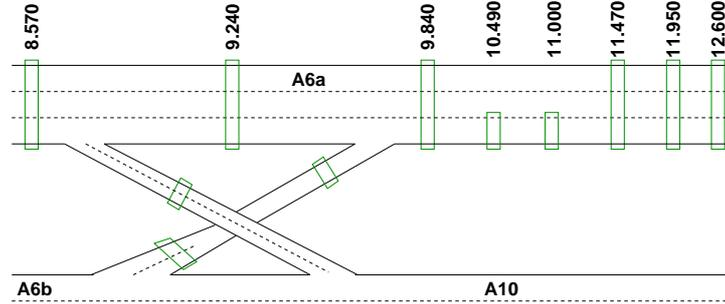
Figure 3: Site A6/A10. Schematic representation of the exchange ramps between highways A6a and A6b and of the inductive loops locations (indicated by rectangles). Vehicles are driving from left to right. The scale is not respected. Only the left lane of highway A6b/A10 is represented.
