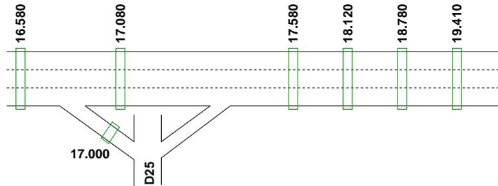
Figure 1: Site A6/D25. Schematic representation of the highway A6 and the on-ramp from D25. Inductive loops locations are indicated by rectangles. Vehicles are driving from left to right. The scale is not respected.
